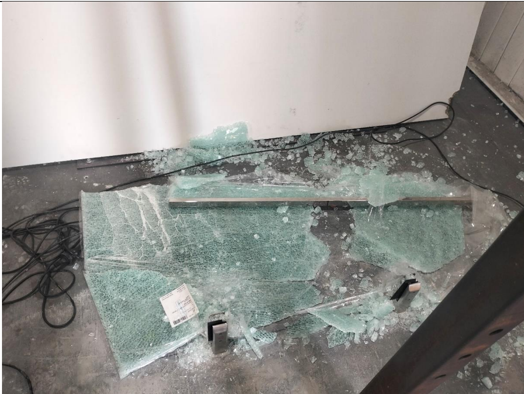
Figure 4: View of typical failure mode for test items 01 and 02.
