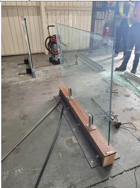
Figure 4: View of typical failure mode for test items 01 through 03, the NANORAIL separated from the glass panel.
