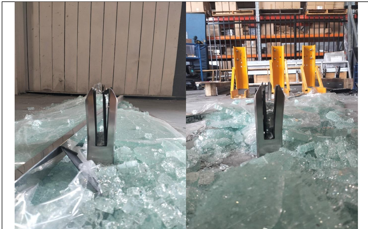
Figure 5: View of permanent deformation of the spigot after the load was released for sample item 01.
