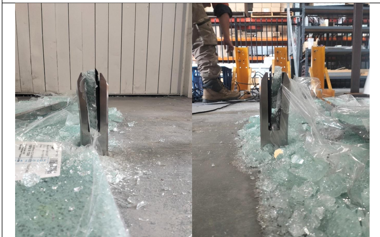
Figure 6: View of permanent deformation of the spigot after the load was released for sample item 02.
