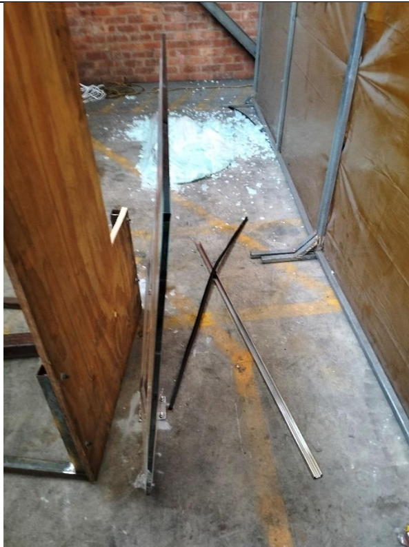
Figure 4: View of typical failure mode for test items 01 and 02, the handrail separated from the glass panel.
