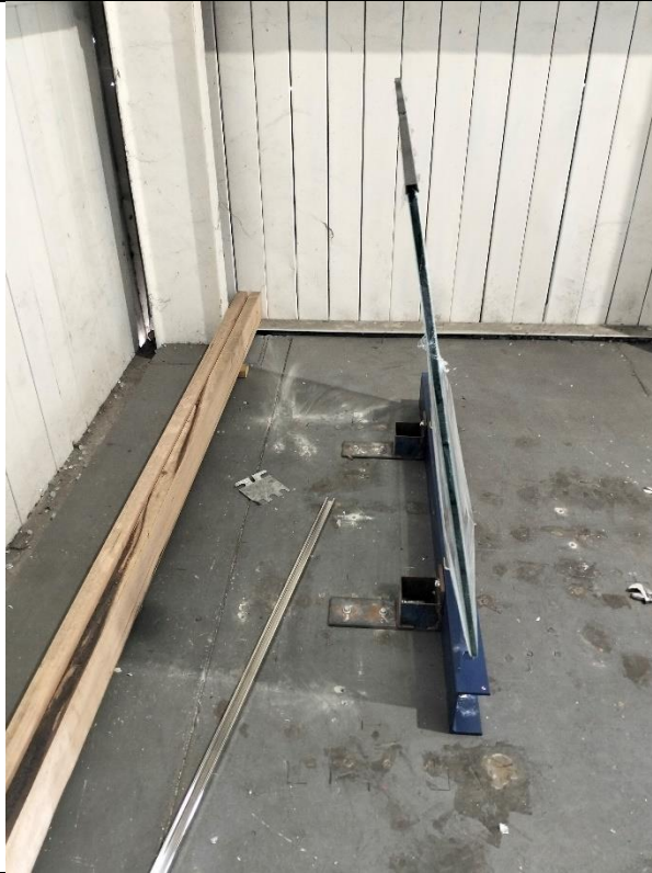
Figure 5: View of the failure mode for test item 03, handrail separated from the glass panel.
