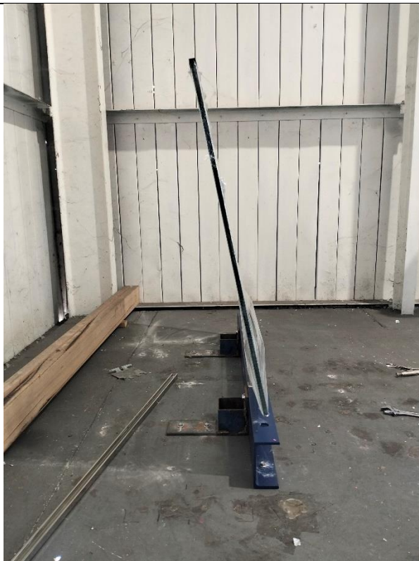
Figure 6: View of permanent deformation of sample item 03 after the load was released.
